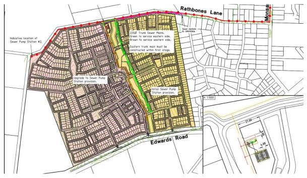
70. The works proposed include a main pumping station (with provision for a second) and 225mm trunk sewer main along Rathbones Lane and Monsants Road to a connection to existing trunk at the Calder Highway.
